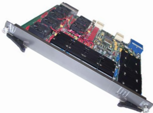
AXIe Compatible Instrument with 12 Independent Channels
